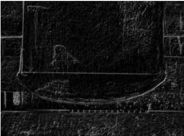
Fig. 2. Output of the Sobel filter - combination of filtering in horizontal and vertical axis.
