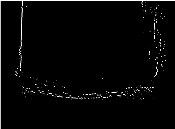
Fig. 6. The output of the search for points that are probably laying on the metal sheet contour.
