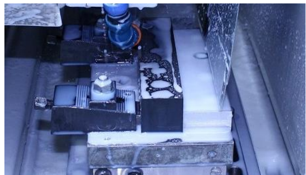
Fig. 9. An example of measuring cutting forces and power with Kistler dynamometr ( v_c=35 m/s, f=200 mm/min, a_p=1,5 mm)
