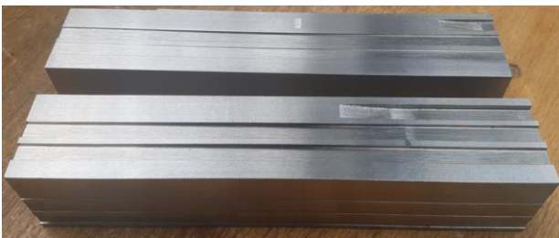
Fig. 14. Workpieces with grooves after creep-feed grinding
