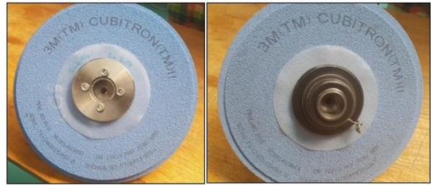
Fig. 6. Cubitron™ II 99% 240x15x50,8 mm 99DA54/80 F15VPLF901W (left) and Cubitron™ II 30% 240x15x50,8 mm 93DA80/80 H15VPMF601W (right)
