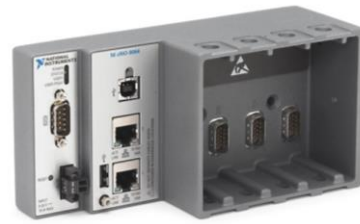
Fig. 9. Control computer cRIO-9064 [12]
