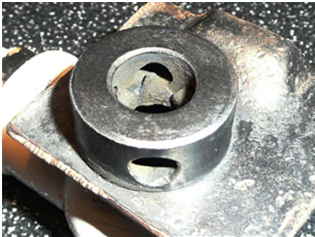
Fig. 1. Distance ring with 4 radial holes [2]
