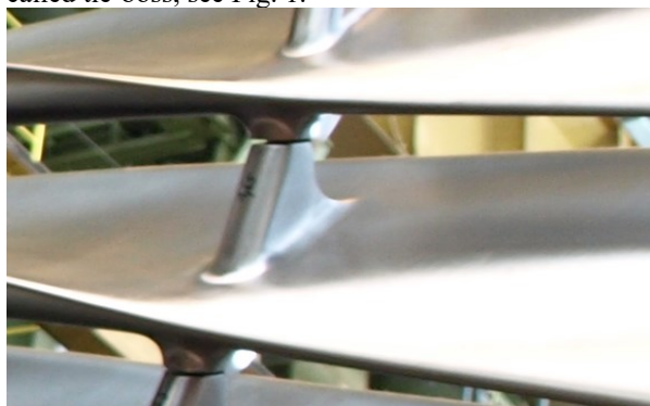
Fig. 1 – Tie-boss mounted on a 1220 mm long blade
