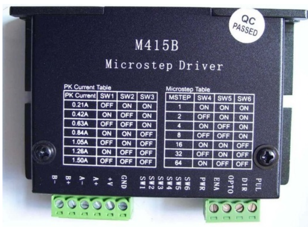
Figure 7: Microstep Driver M415B
