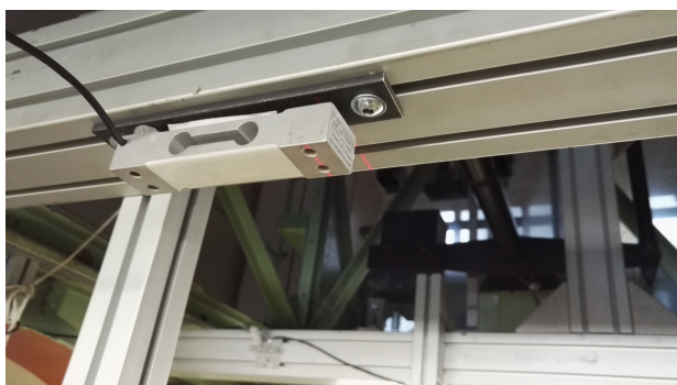
Figure 8: Zemic load cell model L6D, measurement of position by planar laser.
