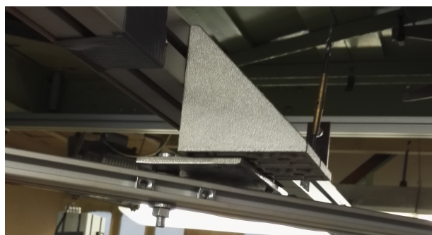
Figure 5: Connective plate, which enables to set different angle of side attack up
