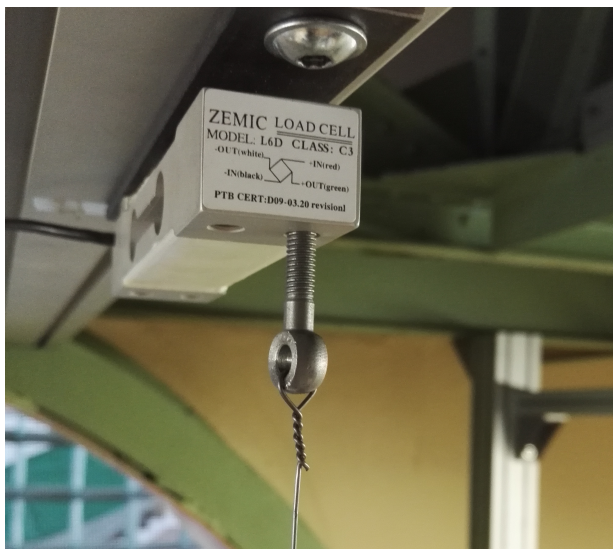
Figure 9: Connection of loading cell with hinge for calibration
