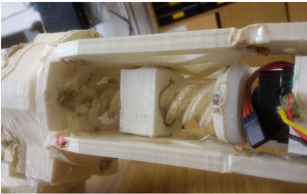
Pic. 5. a worm gearing assembly after repairs.
