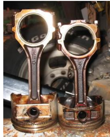
Fig. 18. An example for different length of the connecting rod and piston height (8)
