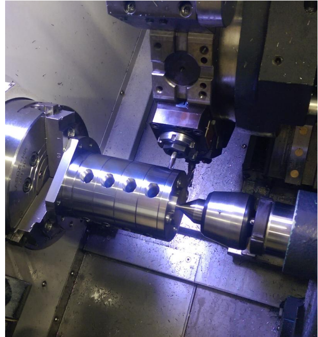
Fig. 4. Modular nut cutting by a CNC machining centre.
