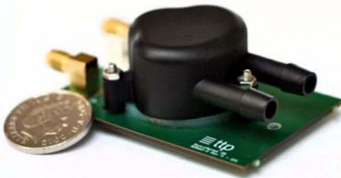
Figure 3. Speed of sound sensor for gas phase [10]
