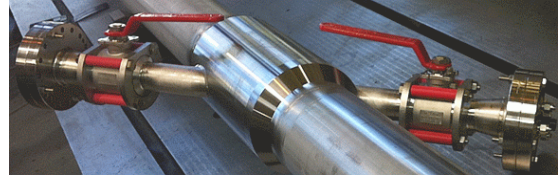
Figure 4. Custom-made ultrasonic flowmeter [11]
