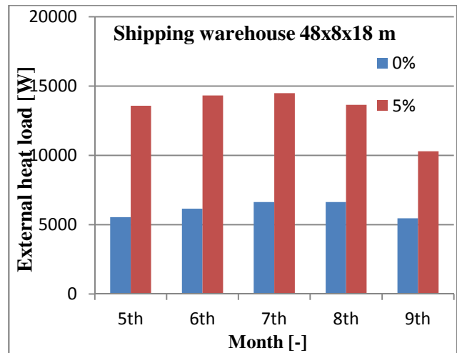
Fig. 7. External heat load for shipping warehouse
