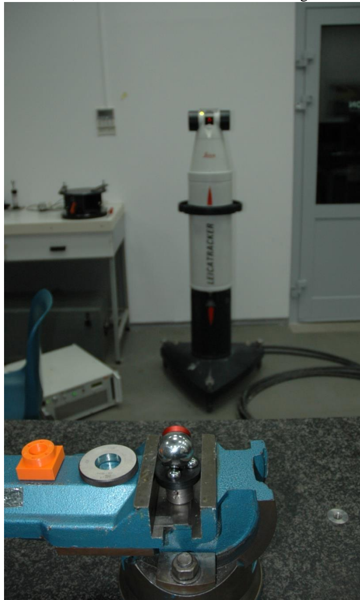
Fig. 3. Measurement station which fixed 1,5 inch retroreflector during measurements.
