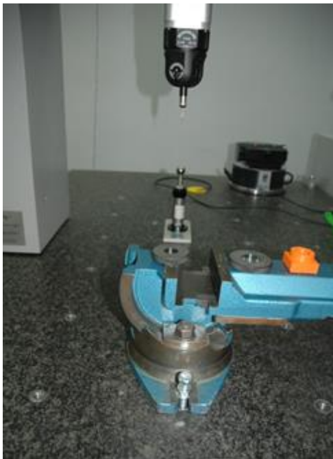
Fig. 2. The experiment setup, the standard mounted in a holder in first position, PH20 probe head
