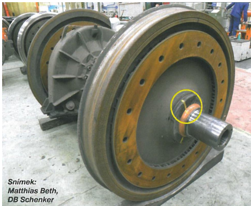
Fig. 7. Wheelset – press-fit slippage, [3]
