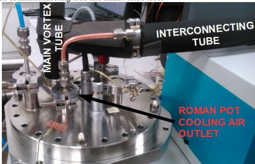
Figure 11: Detail of connection of Roman Pot and interconnecting tube
