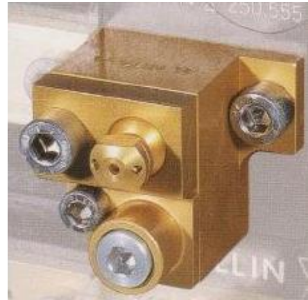
Figure 11. Nozzle of a spraying system
