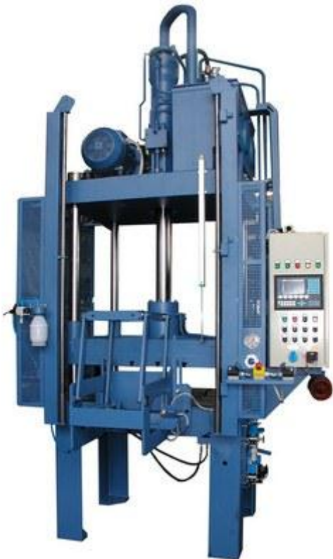
Figure 15. Trimming press from TOS Rakovnik OL28 (280 kN)
