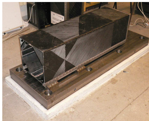
Fig. 2. Hybrid ram with a composite base and steel reinforcements
