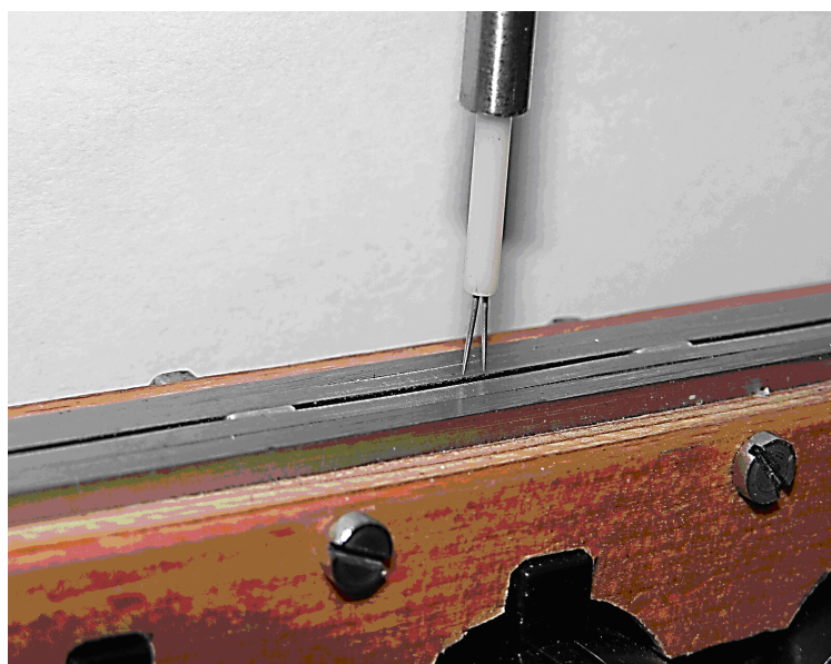
Fig. 4. HWA probe positioning, outlet of the synthetic jet generator
