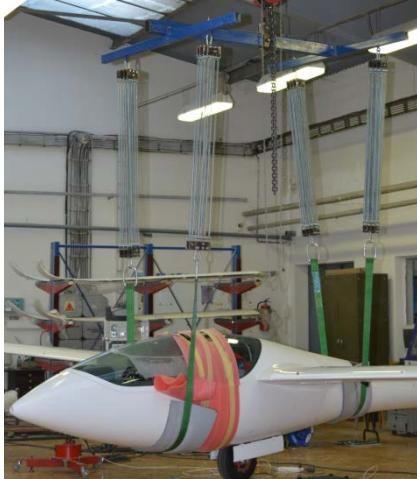
Fig. 9- Frame with very soft springs for sailplanes
