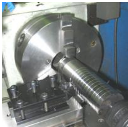
Fig. 1. Machined workpiece made of X165CrV12 mounted in the chuck of machine tool.
