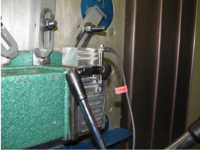
Picture 5 Measurement of cut surface by use of Tesa LVDT displacement sensor
