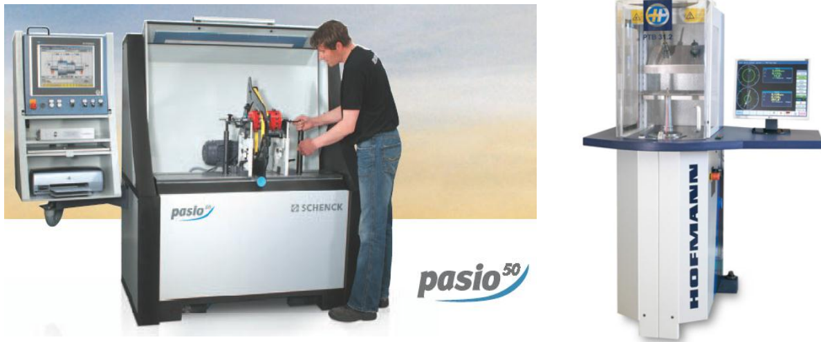
Picture 1 Balancing machine for common use and a specialized balancer for tool holders
