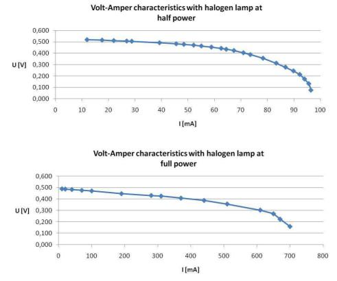
Fig. 9. V-A characteristics of solar cell. Used lamp – halogen 12V 50W. Conditions – darkened room with 0 voltage when lamp turned off. Vertical distance from top of solar cell is 75 mm. Resistance changed from  $0,07\Omega$  to  $39,8 \Omega$ . Top – nominal supply voltage of halogen lamp at half (P=18W). Bottom –lamp voltage at full nominal value (P=50W).
