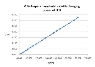
Fig. 12. V-A characteristics of solar cell. Used lamps – 2 high power LED (one with 1.6V), white lamp. Conditions – darkened room with 0 voltage when LEDs turned off. Vertical distance from top of solar cell is 5 mm. Voltage on LEDs changing from bottom value to top value (nominal voltage). Used electrical resistance in circuit is 5,2  $\Omega$ . Solar cell inner electrical resistance is equal to 0,2  $\Omega$ .
