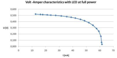
Fig. 10. V-A characteristics of solar cell. Used lamps – 2 high power LED (one with 1.6V), white light. Conditions – darkened room with 0 voltage when LEDs turned off. Vertical distance from top of solar cell is 5 mm. Resistance changed from  $0,07\Omega$  to  $39,8 \Omega$ . Both LED at nominal values of voltage.
