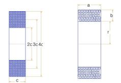
Fig. 16.Brooks coil (left), Cross-wound coil (right)
