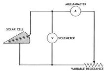
Fig. 8. Method of testing solar cell V-A characteristic [1]
