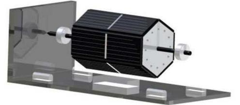
Fig. 14. Concept of Mendocino motor – motor is levitating above 2 neodymium magnets, which are replacing the bearings for no friction. Function of central neodymium magnet is described in Fig. 14. Because of opposite poles of neodymium magnets, motor is pushed towards the wall, making it stable in one position. There are several upgrades that can be made to improve its performance, such as adding more magnets and lamps around to create higher voltage on solar cells.
