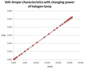
Fig. 13. V-A characteristics of solar cell. Used lamp – halogen 12V 50W. Conditions – darkened room with 0 voltage when lamp turned off. Vertical distance from top of solar cell is 75 mm. Voltage on halogen lamp changing from bottom value to top value (nominal voltage). Used electrical resistance in circuit is 20  $\Omega$ . Solar cell inner electrical resistance is equal to 0,2  $\Omega$ .
