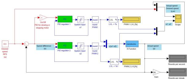
Fig. 17. Simulink model for controlling Mendocino motor
