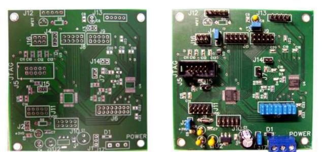
Fig. 4. Unassembled PCB (left), assembled PCB (right)
