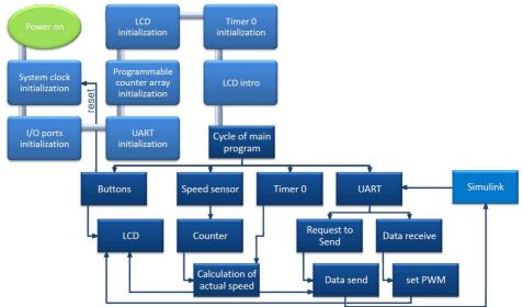
Fig. 17. Simplified flowchart of program in control unit. Cycle of main program is in loop, for simplicity some side-steps are not shown. Program ends with turning control unit off.
