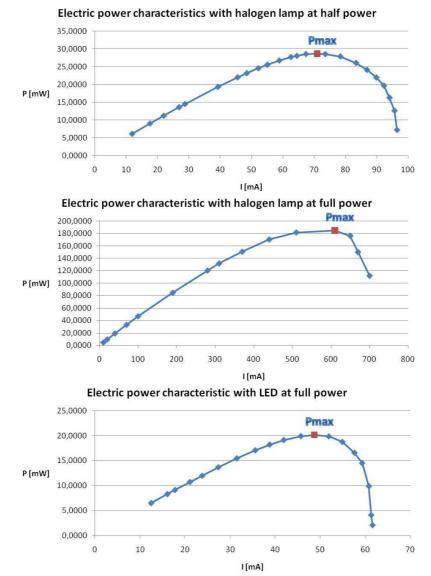
Fig. 11. Electric power characteristics of solar cell for previous settings from Fig. 9 and 10. Top – Pmax=28,643 mW, U=0,403 V, I=71 mA; middle - Pmax=184,83 mW, U=0,303 V, I=610 mA; bottom- Pmax=20,162 mW, U=0,414 V, I=48,7 mA
