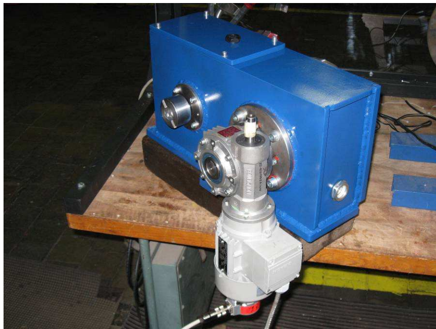
Fig9. Planetary gear controlled by servo motor
