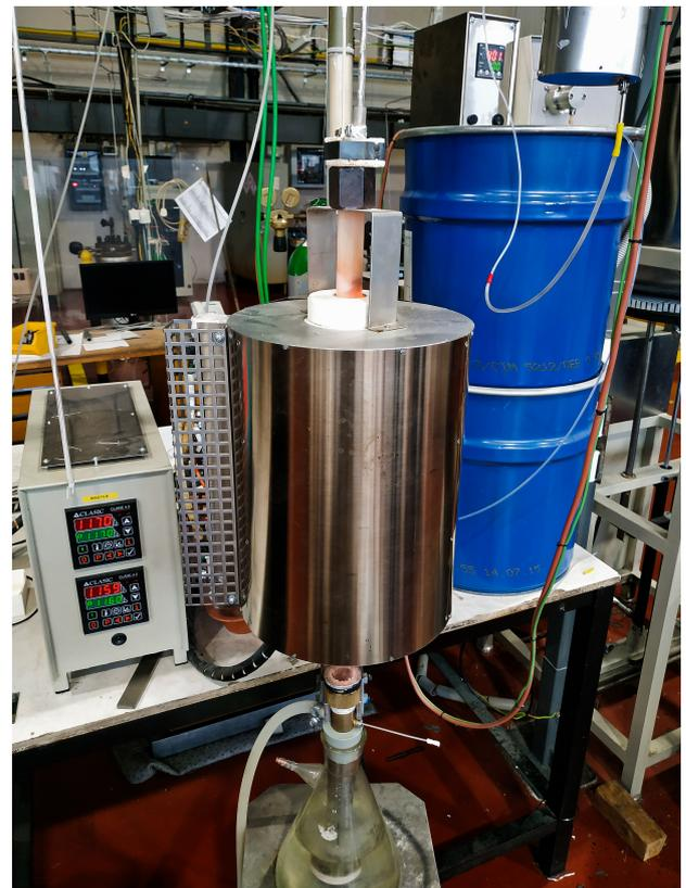
*Fig. 4. The apparatus for high-temperature oxidation.*
