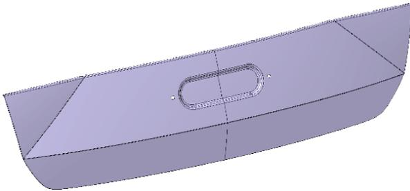
**Figure 11.** ŠKODA RAPID SPACEBACK (2012), fifth door outer rear.
