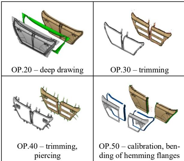
Figure 2. ŠKODA FABIA, CAD data of tools.
