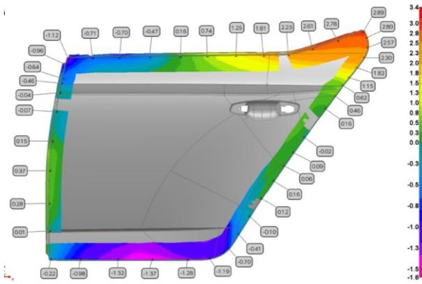
Figure 6. Springback measurement result, HX180BD.
