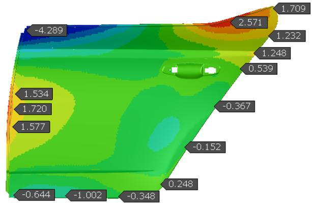
Figure 8. Springback in normal direction, DP500, MTC 1.
