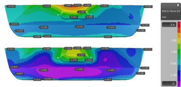
**Figure 15.** Virtual springback in normal direction, DC05 (above) and DP500 - MTC 1 (below).
