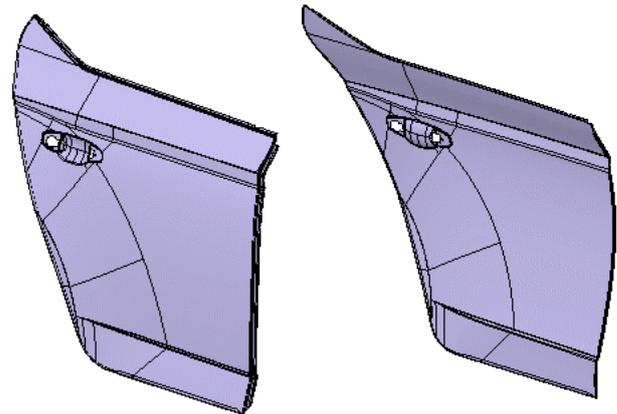
**Figure 1.** ŠKODA FABIA III (2014), side door outer rear.
