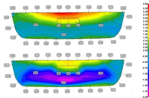
**Figure 14.** Virtual springback in normal direction, DC05 (above) and DP500 - MTC 1 (below).
