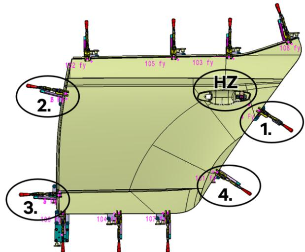
Figure 5. ŠKODA FABIA, Position of RPS points (clamps).
