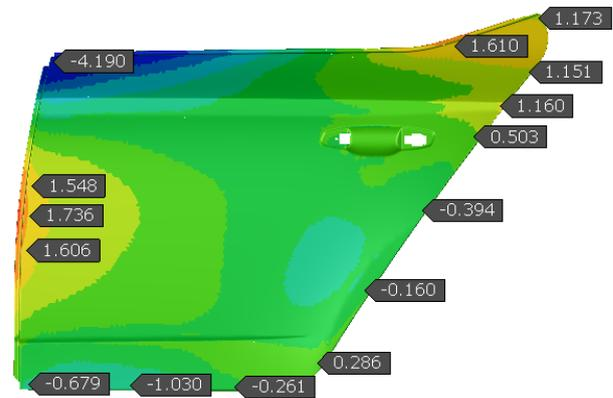
Figure 9. Springback in normal direction, DP500, MTC 2.
