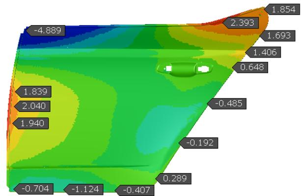
Figure 10. Springback in normal direction, DP500, MTC 3.
