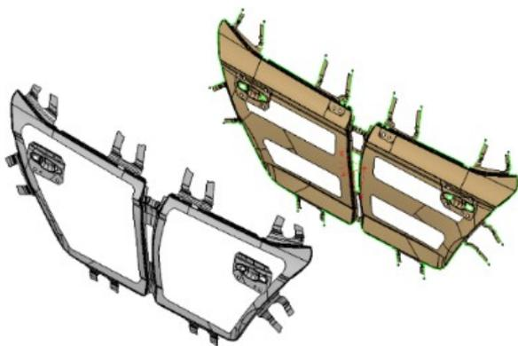
Figure 3. Pad (gray), Post (brown) and Cutting Curves (green) in OP.40 (Trimming and Piercing).
