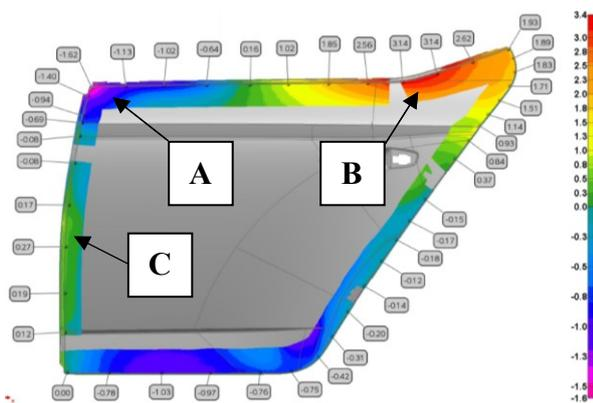
Figure 7. Springback measurement result, DP500.
