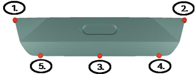
**Figure 13.** ŠKODA RAPID SPACEBACK, Position of RPS points (clamps).
