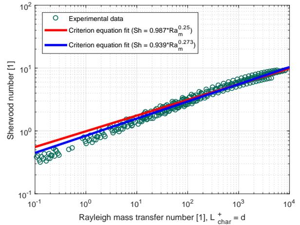
**Fig. 4.** Mass transfer results: Sherwood number correlation, Rayleigh number based on  $L_{char} = d$ . Experimental data are fitted by two criterion equations
