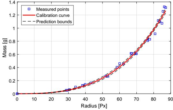
**Fig. 2.** Calibration curve for mass evaluation from thermograms
