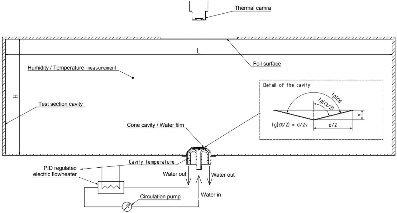
**Fig. 1.** Schematic diagram of the experimental apparatus:  $L = 1\text{m}$ ,  $H = 0.3\text{m}$ ,  $B = 0.3\text{m}$  (width); water film is observed by thermal cam, the cavity is maintained at steady temperature by outer water circuit. In the dashed box is geometrical description of the cavity
