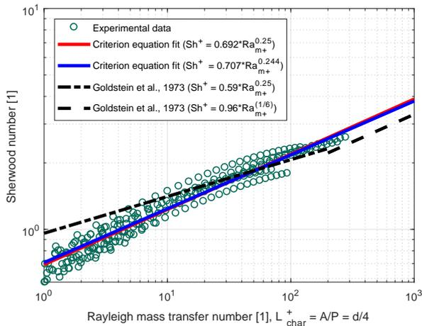
**Fig. 5.** Mass transfer results: Sherwood number correlation, Rayleigh number based on  $L_{char} = d/4$ . Experimental data are fitted by two criterion equations and compared with correlations from reference [4]
