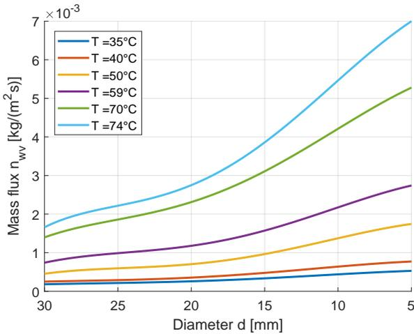
**Fig. 3.** Mass transfer results: dependency of mass flux  $n_{wv}$  on film diameter and film temperature
