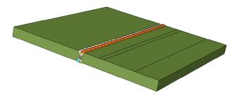
Fig. 4. The Partition model, green is base metal, each one of beads is colored and is divided into 28 chunks.
