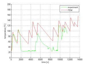
**Fig. 6.** The temperature development at place, where one of the thermocouples was installed.
