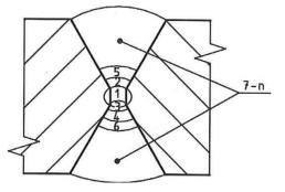
Fig. 2. Structure of welding beads.
