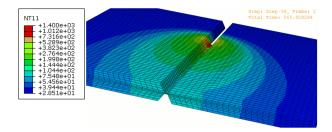
Fig. 5. The temperature distribution, when first bead is being added.
