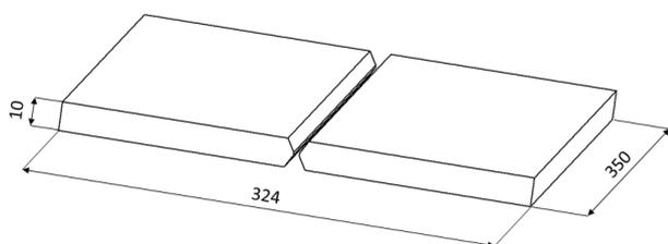
*Fig. 1. Scheme of welded plate with dimensions.*
