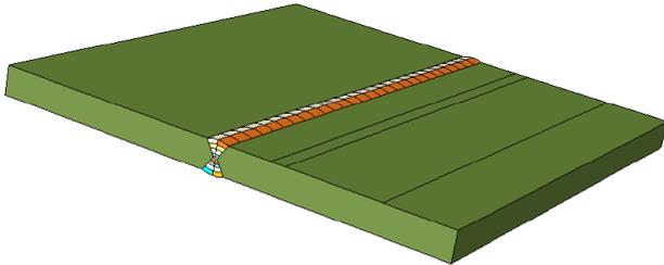
**Fig. 4.** The Partition model, green is base metal, each one of beads is colored and is divided into 28 chunks.
