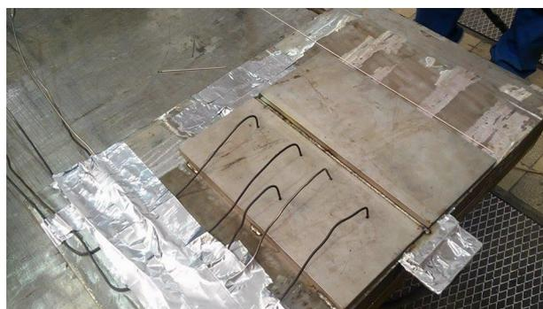
*Fig. 3. Installation of thermocouples on specimen surface.*
