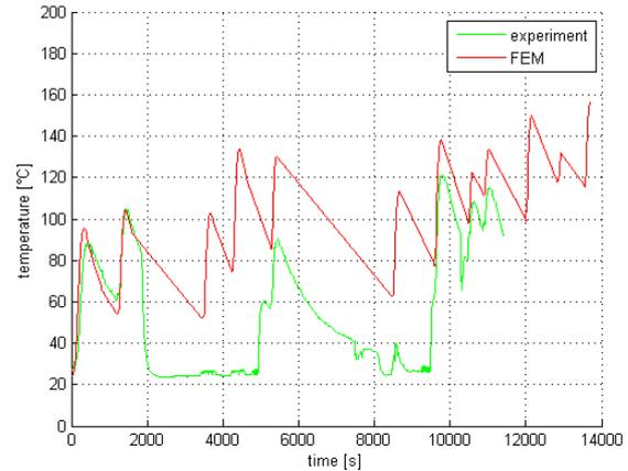
**Fig. 6.** The temperature development at place, where one of the thermocouples was installed.
