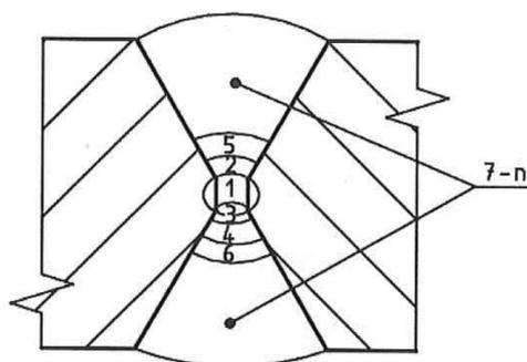
*Fig. 2. Structure of welding beads.*
