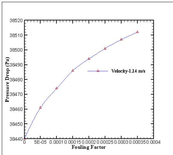
Figure 8: fouling factor vs pressure drop at 1.14 m/s velocity
