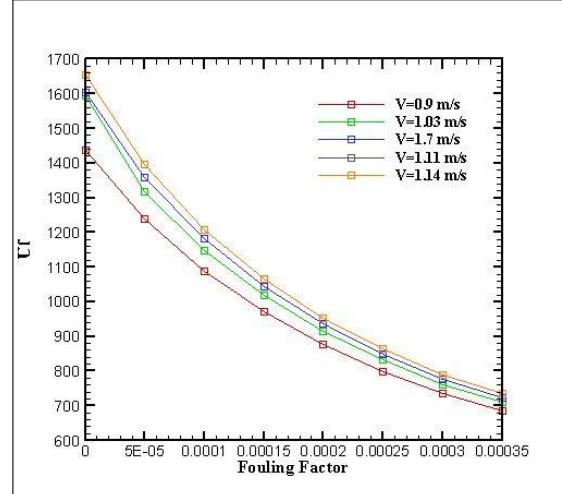
Figure 10: Fouling Factor vs  $U_f$
