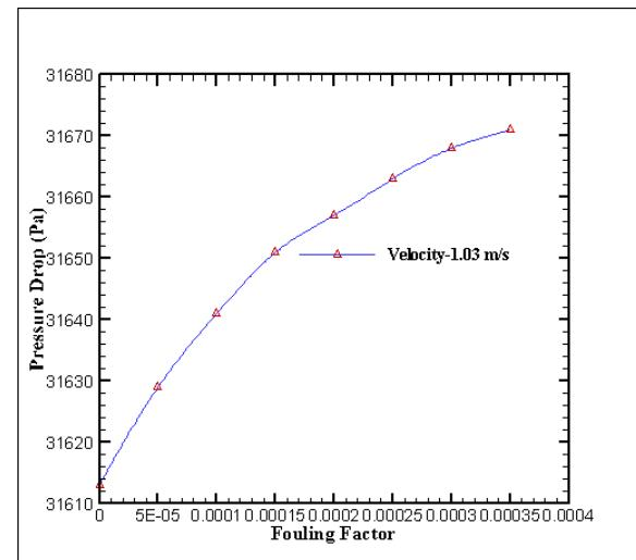
Figure 5: fouling factor vs pressure drop at 1.03 m/s velocity
