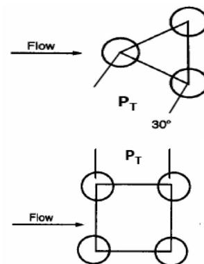
Figure 3: Square and Triangular Pitch Tube Layout<sup>[17]</sup>
