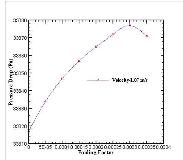
Figure 6: fouling factor vs pressure drop at 1.07 m/s velocity
