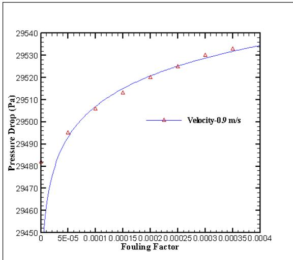
Figure 4: fouling factor vs pressure drop at 0.9 m/s velocity
