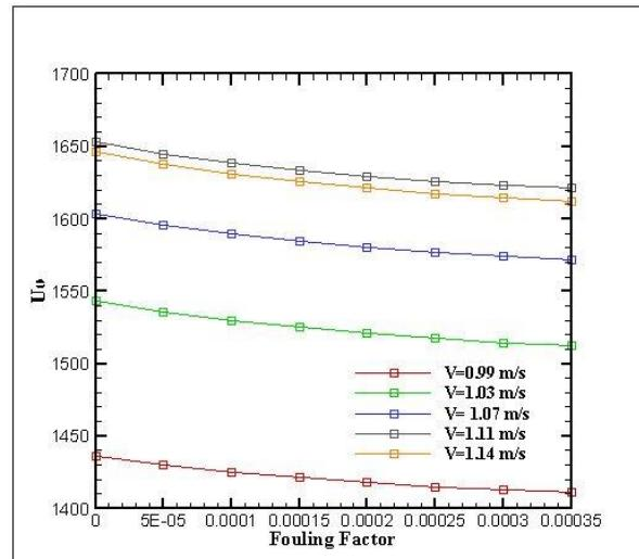
Figure 9: Fouling Factor vs  $U_o$
