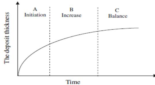
Figure 1: the deposition thickness<sup>[2]</sup>
