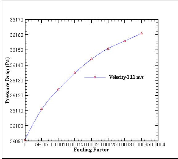
Figure 7: fouling factor vs pressure drop at 1.11 m/s velocity
