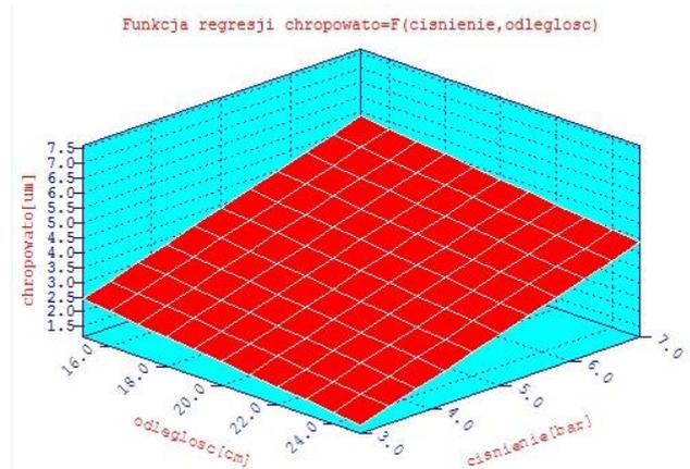
Figure 5 Roughness of the surface depending on the distance of nozzle and pressure for angle of 30°
