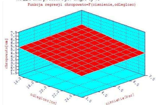
Figure 7 Roughness of the surface depending on the distance of nozzle and pressure for angle of  $60^\circ$
