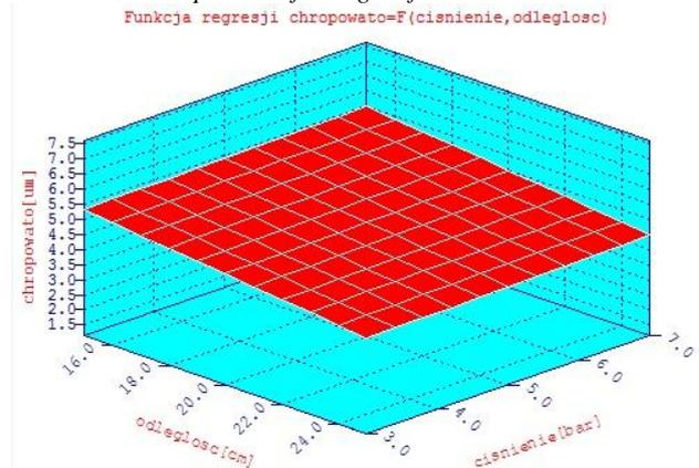
Figure 7 Roughness of the surface depending on the distance of nozzle and pressure for angle of 60°
