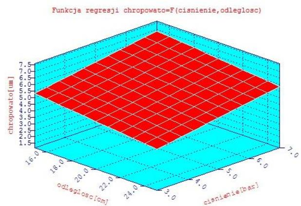
Figure 6 Roughness of the surface depending on the distance of nozzle and pressure for angle of  $45^\circ$
