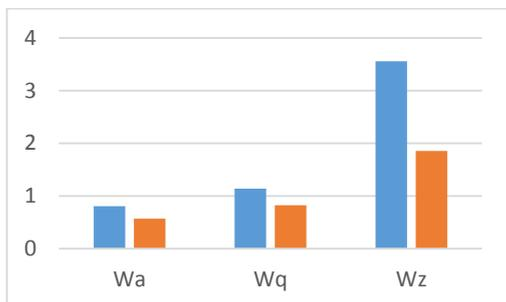
Figure 10 The chart shows the relationship between waviness parameter and their value. The blue color represents the values measured perpendicularly to the longer edge of the sheet, and color orange represents measurements parallel to the longer edge.
