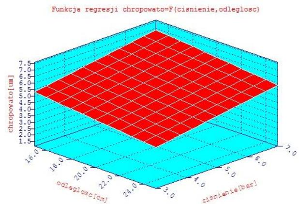
Figure 6 Roughness of the surface depending on the distance of nozzle and pressure for angle of 45°
