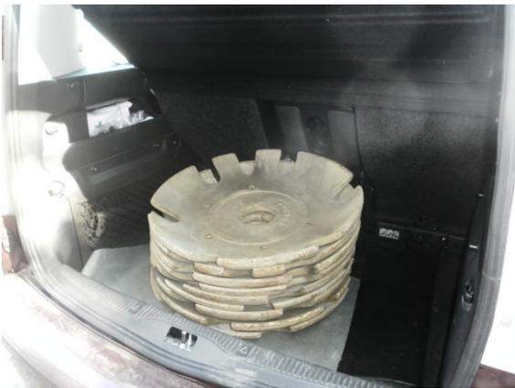
Fig. 2 Cast iron weights wheeled tractor 10 pieces 1 piece has a weight of 43 kg.
