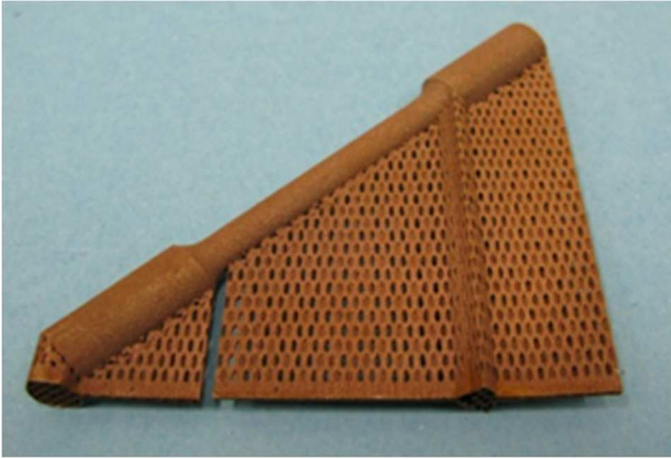
Fig. 3. Tensile test bar printed under 45° angle before breaking away the supports – surface discoloration after annealing.
