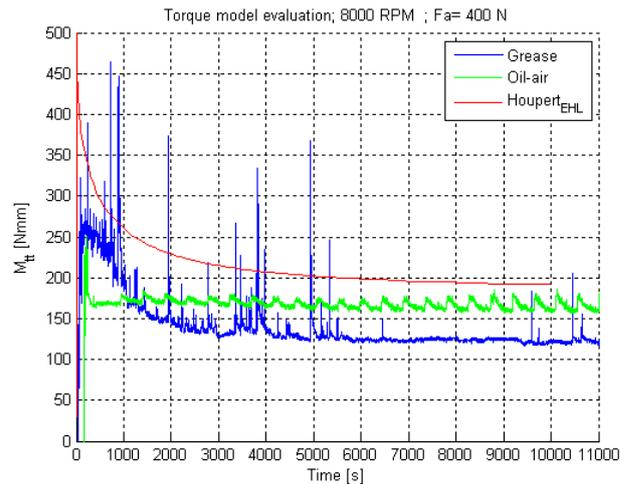
**Fig. 10.** Comparison of measured data and simulation model 8000 RPM, 400 N axial preload, oil-air and grease lubrication; FAG B7214-C-T-P4S
