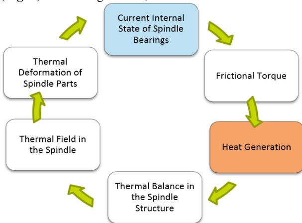
Fig. 3. Closed loop of thermal effect in spindle bearings.
