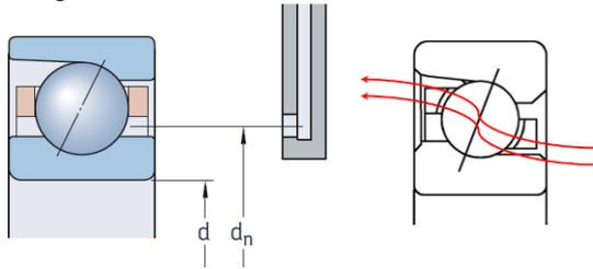
**Fig. 8.** Supply oil-air to the bearing [16]
