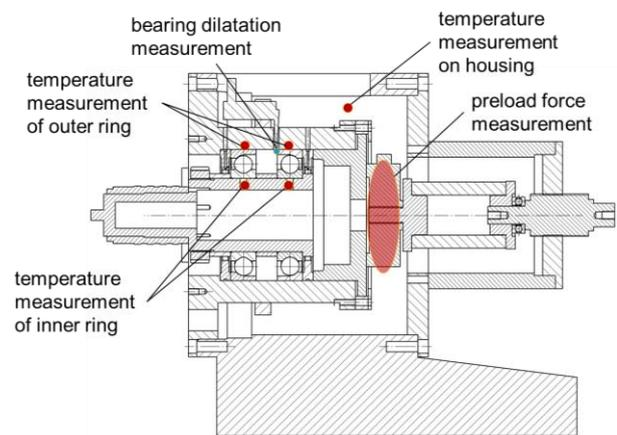
Fig. 6. Measurement of test rig
