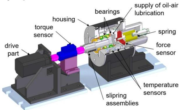
Fig. 4. Test rig main components.
