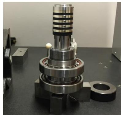
Fig. 7. Sliping assemblies for temperature measurement of spindle bearing inner rings
