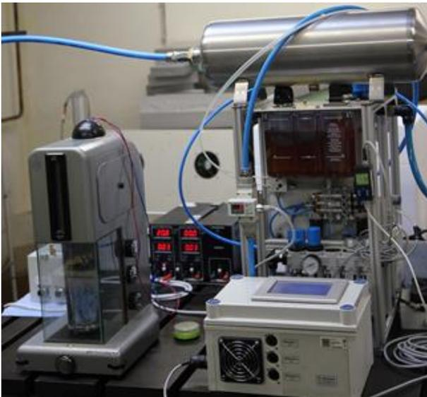
**Fig. 9.** Oil – air lubrication unit
