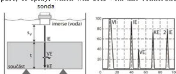
**Fig. 1.** Arrangement in immersion testing, VI – a pulse, IE – interface echo, KE – back wall echo
