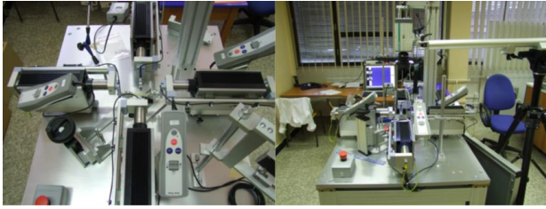
Figure 1: Biaxial testing machine for soft tissue and elastomer mechanical testing
