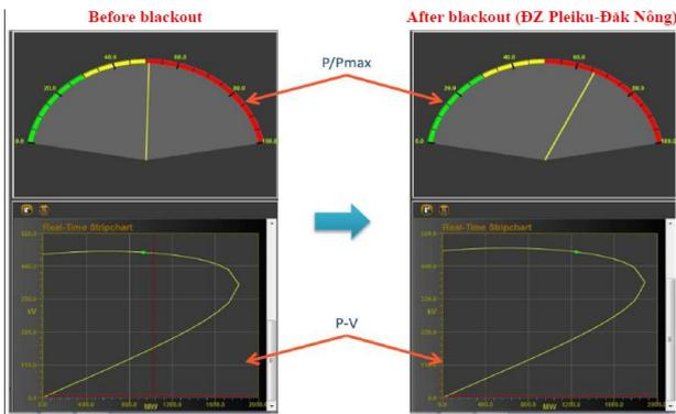
Figure 7. Voltage sensitivity on SmartWAMS
