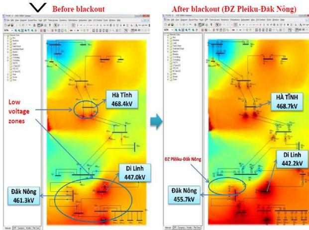
Figure 6. Calculation results on PSS/E when blackouted Pleiku-Dak Nong power line (22 May 2013)
