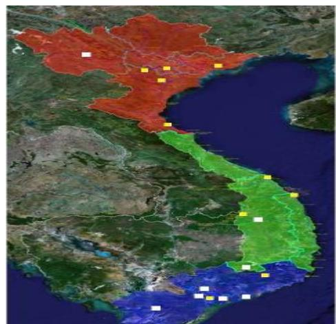
Figure 5. PMU locations in 500kV Vietnam grid
