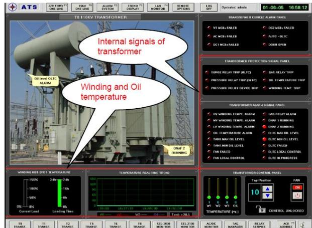
Figure 1. Transformer parameters on display screen
