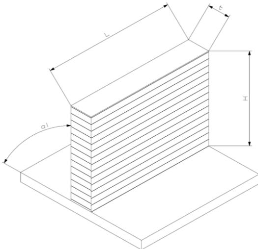
Figure 3. The parametric model of plate with dimension
