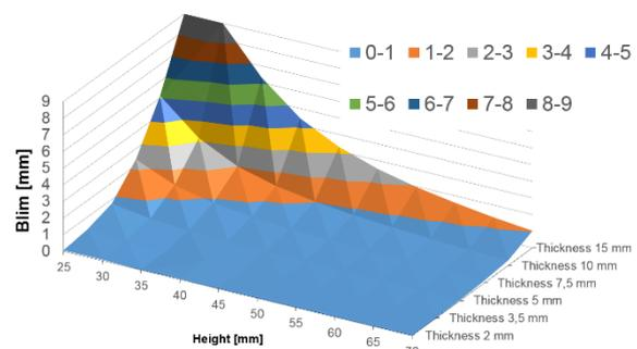
Figure 6 The critical depth of cut for different dimensions of plate
