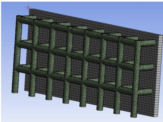
Figure 8. The model of plate with support structures in software ANSYS.
