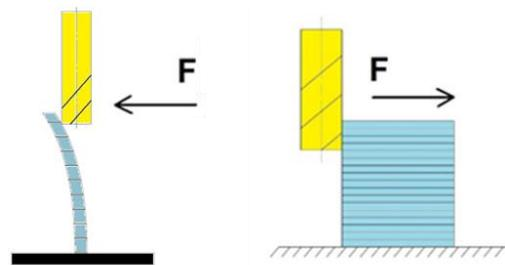
**Figure 2.** Machining of the thick-walled parts in comparison with machining the thin-walled parts
