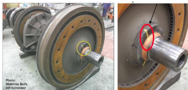
Fig. 2. Wheel disc relative rotation detail [3]
