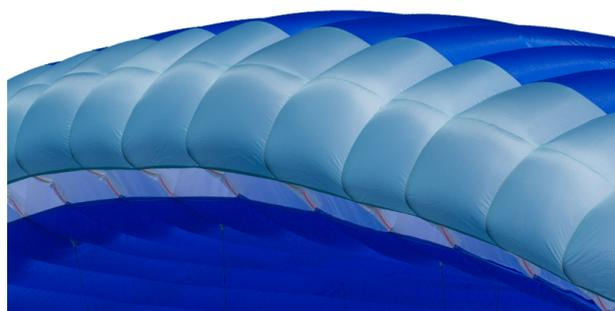
*Fig. 2. Detail of the paraglider intakes.*
