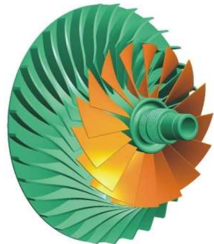
Fig. 1. A study of a tandem-bladed impeller [5]
