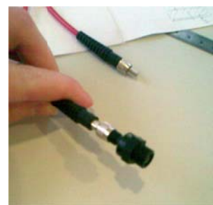
Fig. 5. Collimating lens mounted to a light guide
