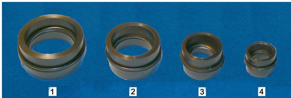
Fig. 5 Shapes of the inner butt welds in the PE pipeline joints 1 - 63 x 5,8; 2 - 50 x 4,6; 3 - 40 x 3,7; 4 - 32 x 2,9
