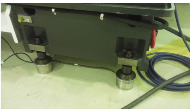
Fig. 16. Leveling bolts with load cells on the machine
