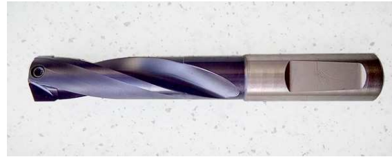
Figure 4. Customized drill bit from Gühring.
