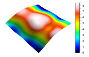
Figure 9 3D image of the waviness of the surface
