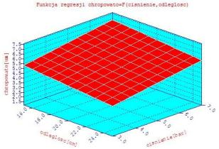
Figure 6 Roughness of the surface depending on the distance of nozzle and pressure for angle of 45<sup>0</sup> Funkcja regresji chropowato=F(cisnienie, odleglosc)
