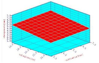
Figure 7 Roughness of the surface depending on the distance of nozzle and pressure for angle of  $60^{\circ}$
