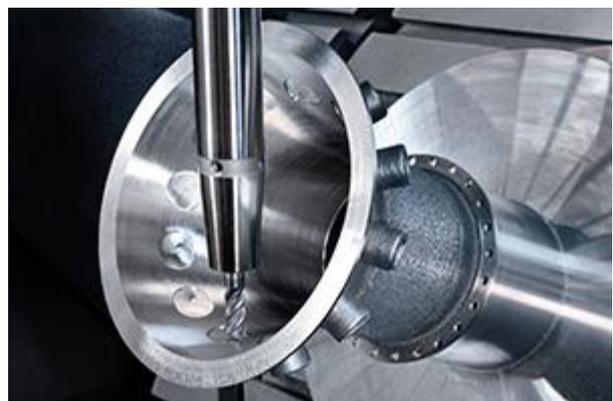
*Fig. 4. Final finish milling [1]*
