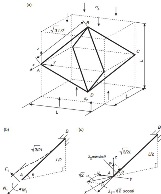
Fig. 7. Geometry of the BCC unit-cell, showing the loading conditions and movement of each strand: (a) geometry of the BCC unit cell, (b) loading conditions, (c) movement of 'A' relative to 'B'. [5]
