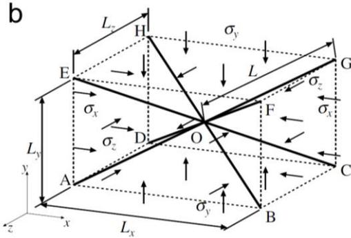
Fig. 8. Geometries and loading condition for a representative unit-cell [6]
