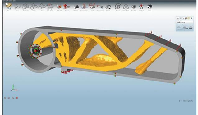
Fig. 11. The optimized distribution of filling materials according to the static load acting on the part [8]
