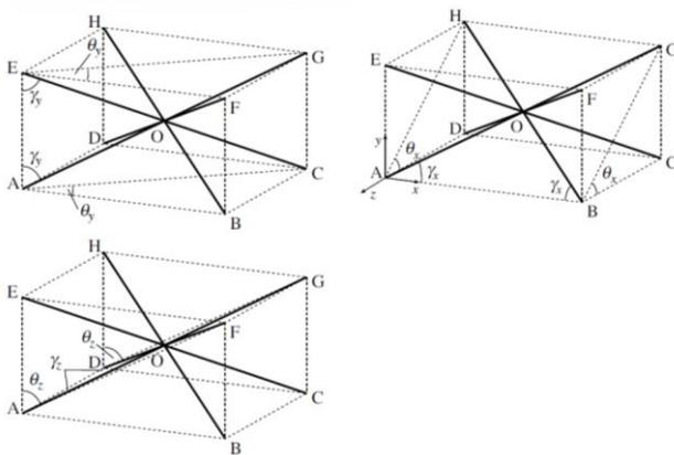
Fig. 9. Definition of angles  $\gamma_x, \gamma_y, \gamma_z$  for a unit-cell. [6]
