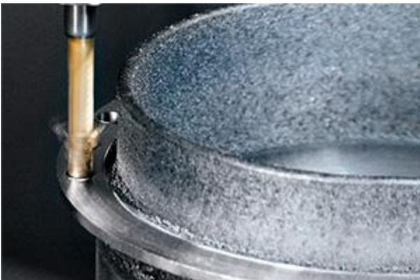
*Fig. 2. Machining between printing [1]*
