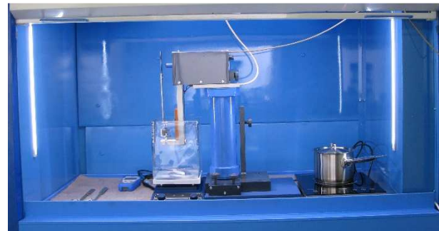
Fig. 2. Residual stress measurement device, CTU
