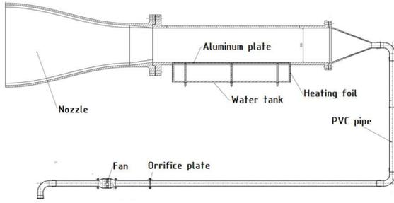
Fig. 3. Test rig design.
