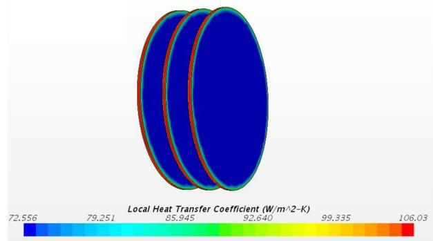
Fig. 8. Values of Local heat transfer coefficient.
