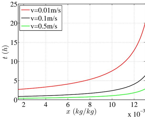
Fig. 6. Time of evaporation dependency on specific humidity for different values of moist air velocity
