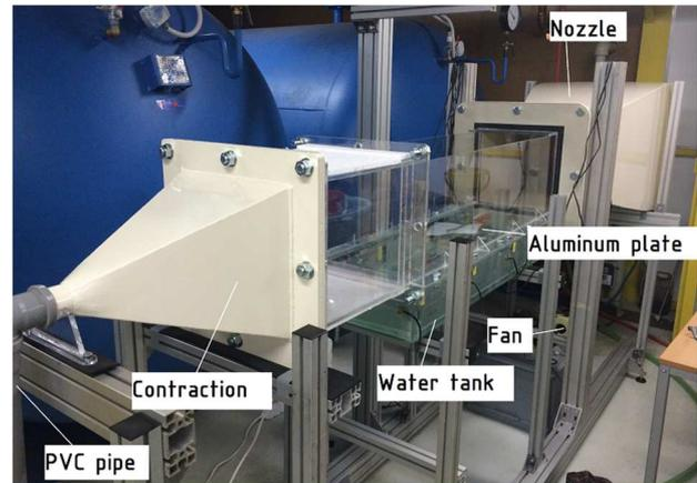
Fig. 5. Picture of the test rig.
