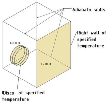
Fig. 2. Geometry of the fluid domain.
