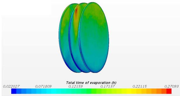
Fig. 12. Total time of evaporation of water film of 0,1mm thickness.
