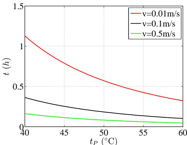
Fig. 7. Time of evaporation dependency on the surface temperature for different values of moist air velocity.
