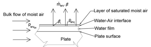
*Fig. 1. Thin water film evaporation scheme.*
