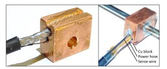
Figure 7. Power terminal connection to stave. Note the connection of power hose and sense-wire.
