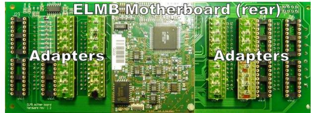
**Figure 9.** ELMB Motherboard (rear side) with mounted ELMB unit and equipped with voltage and resistance adapters.
